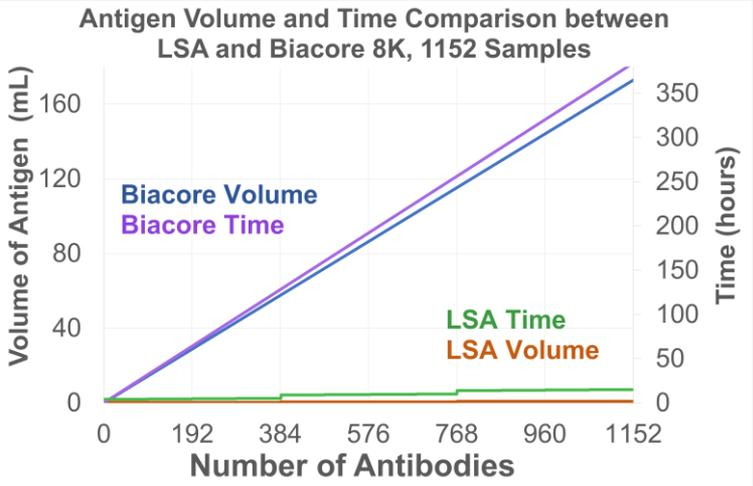
**This represents a capture kinetics assay with equivalent number of injections (7 concentrations + blank) for assay timing on both systems.**
