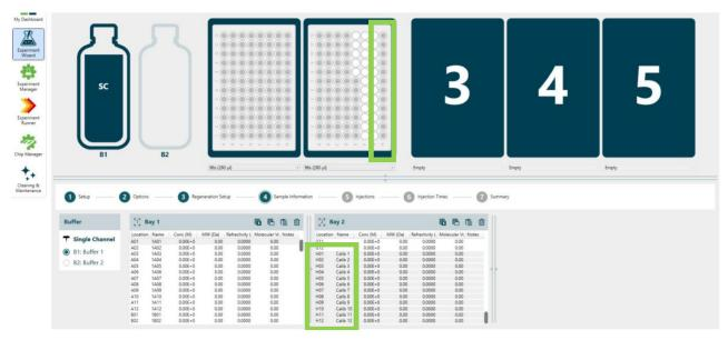
4. Add calibrant solutions to SC injections list at the end of the sample injections.
